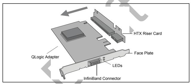
Figure 4-8. QLogic QHT7140 Adapter with Riser Card
